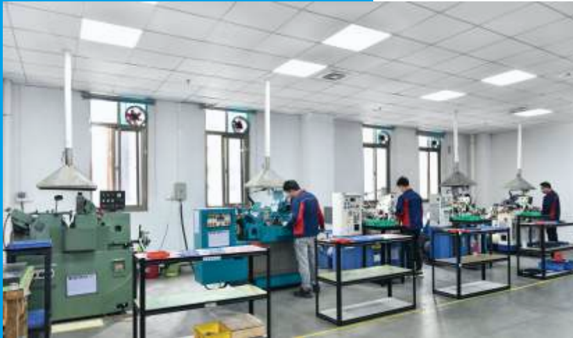
无芯磨车间 Centerless Grinder Operation
